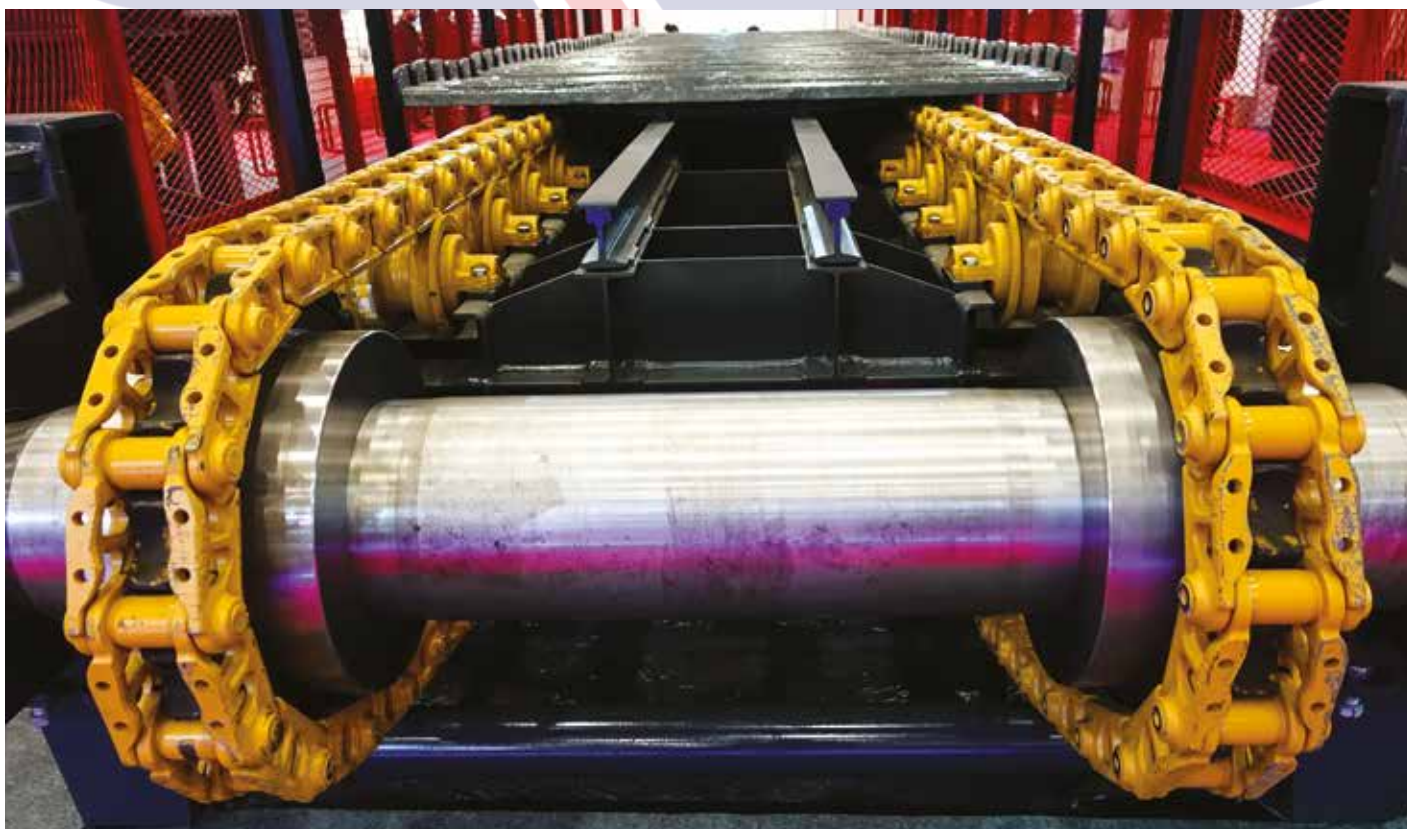
Locking conveyor chain wheels using SIT-LOCK® 4 COMPACT.
