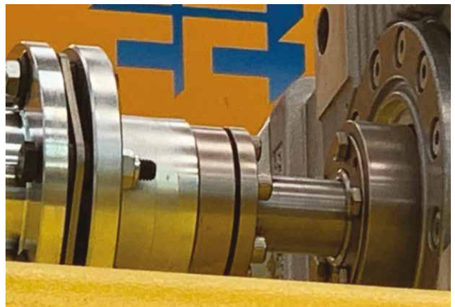
SIT-LOCK® 3 used for a disc coupling.
