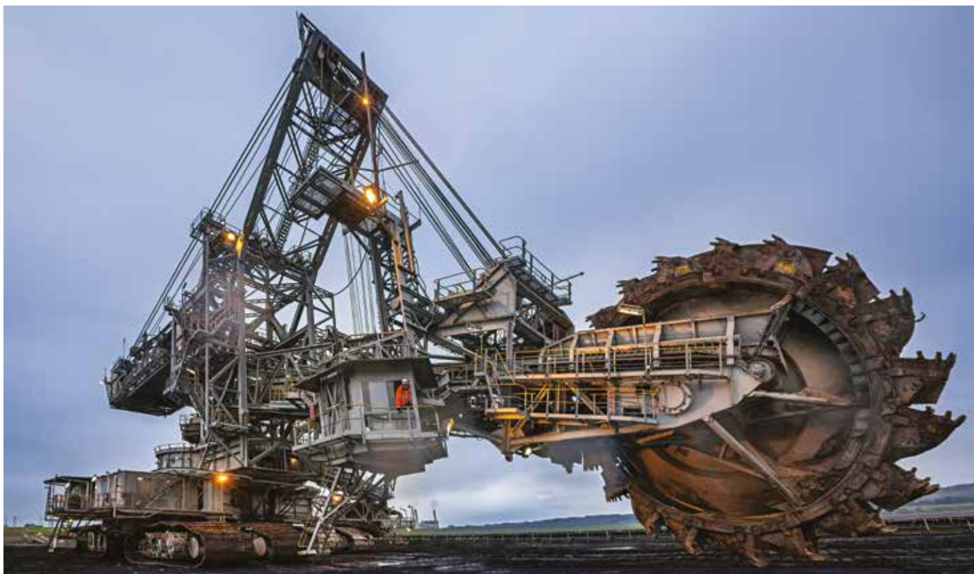
Quarry excavator application: SIT-LOCK® 4 COMPACT for drums and SIT-LOCK® 14 for bucket wheel locking.
