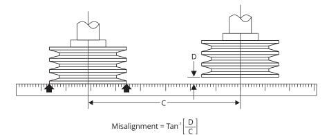
The total allowable misalignment recommended for V-Belts, in general, is 1/2-degree. While individual V-Belts are known to be capable of handling greater amounts of misalignment before becoming unstable, maintaining the misalignment to within 1/2-degree will maximize Belt life.
