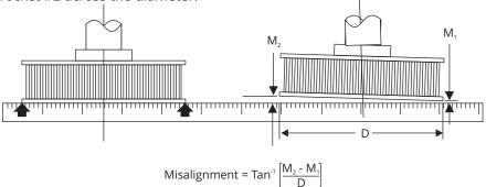
The angle of parallel misalignment can be quantified as the difference in clearance between the straight edge and the outer surfaces of the two sheaves or sprockets across the separation distance.
